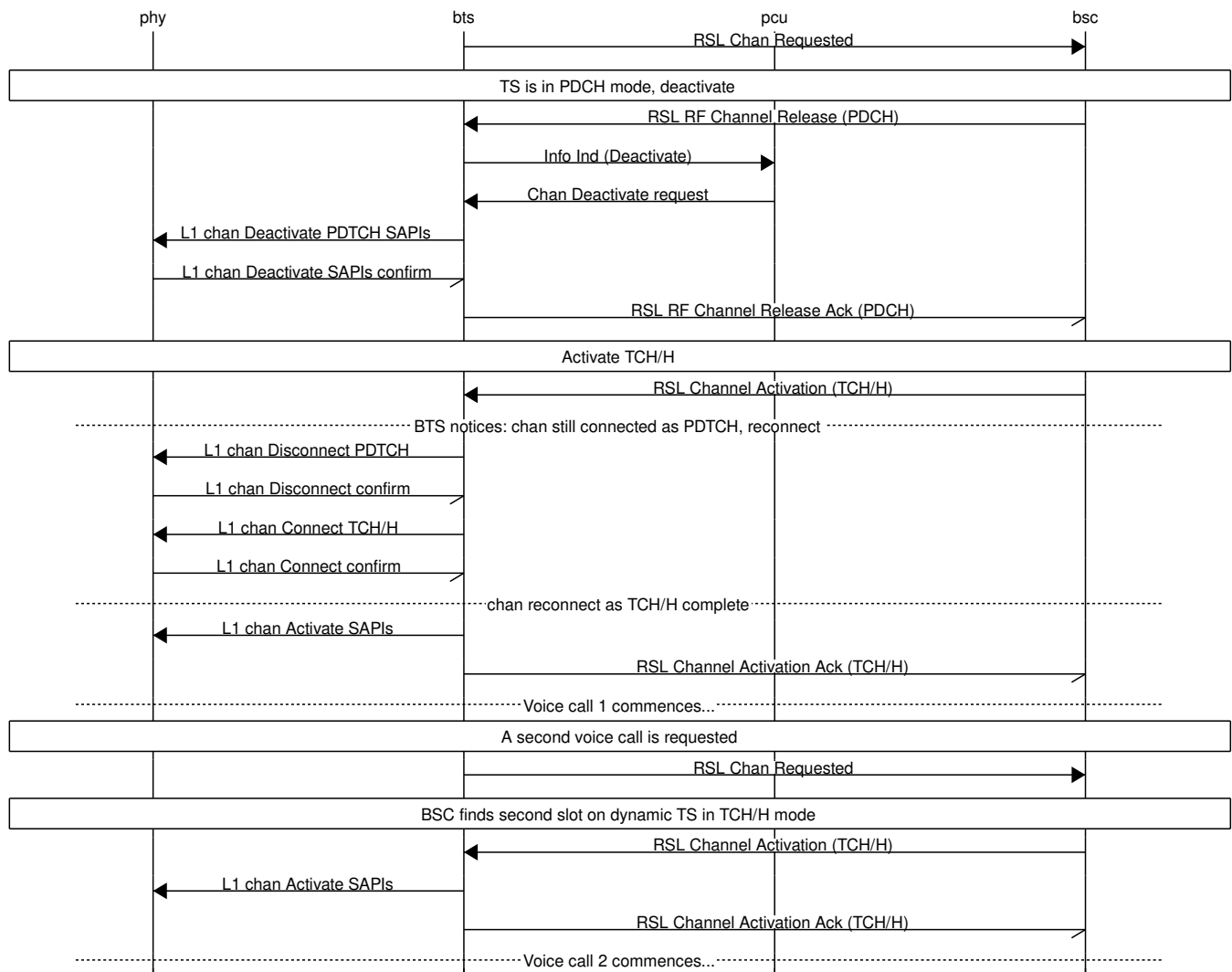
Figure 12: Part 1: example for dynamic channel switchover, for Osmocom style dynamic timeslots
